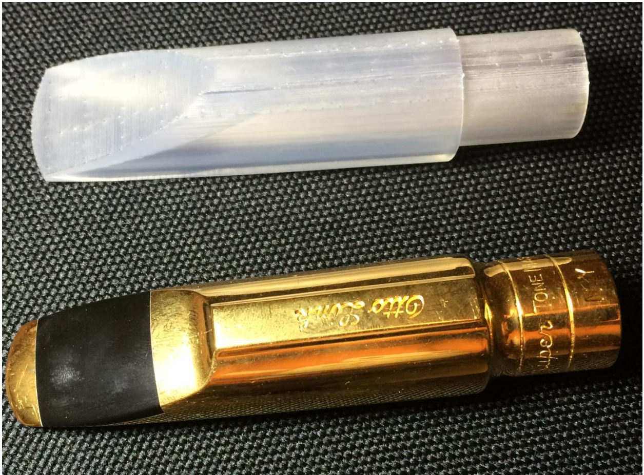
Figure 3: 3D printed mouthpiece next to traditional metal mouthpiece.
